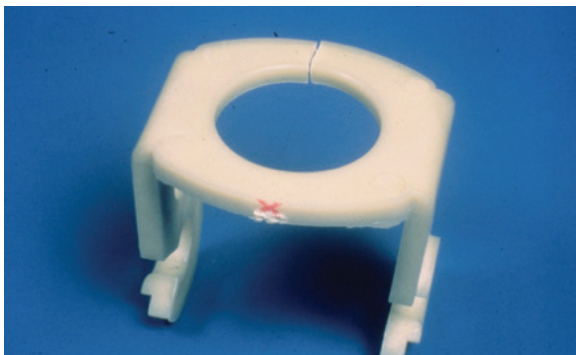
Figure 1. Weld line failure in a glass-filled nylon clevis part
