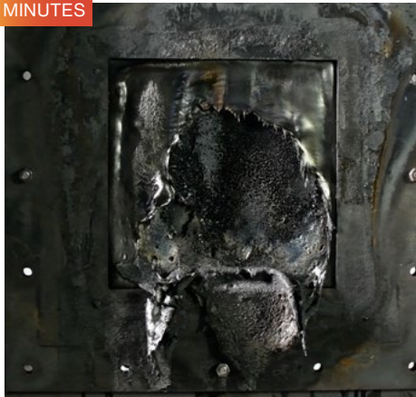
Standard Flame-Retardant PA66 (3mm) Breached in less than 3 minutes
