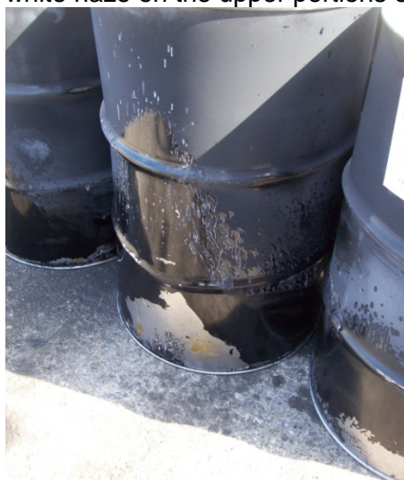
Figure 2 – HMD Carbamate collected on surface of a drum after a nearby spill. HMD Carbamate is the white haze on the upper portions of the drums.
