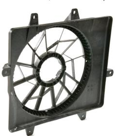
are critical in maintaining the positioning of the fan to the radiator. The natural damping characteristics of Vydyne PA66 help eliminate vibration that leads to NVH issues. Also, the chemical resistance of PA66 eliminates problems with typical automotive chemicals.
